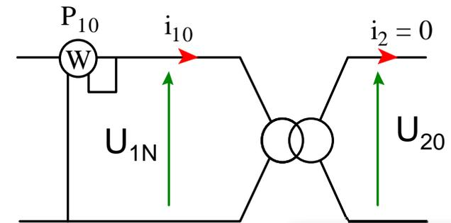
$$Q_{10} = l_1 \omega I_{10}^2 + l_2 \omega I_2^2 + \frac{U_{10}^2}{L_m \omega} \quad \text{or} \quad I_{10} \ll I_{1N} \quad (10\% I_{1N}) \quad \text{et} \quad I_2 = 0 \quad \Rightarrow L_m \omega = \frac{U_{10}^2}{Q_{10}}$$
